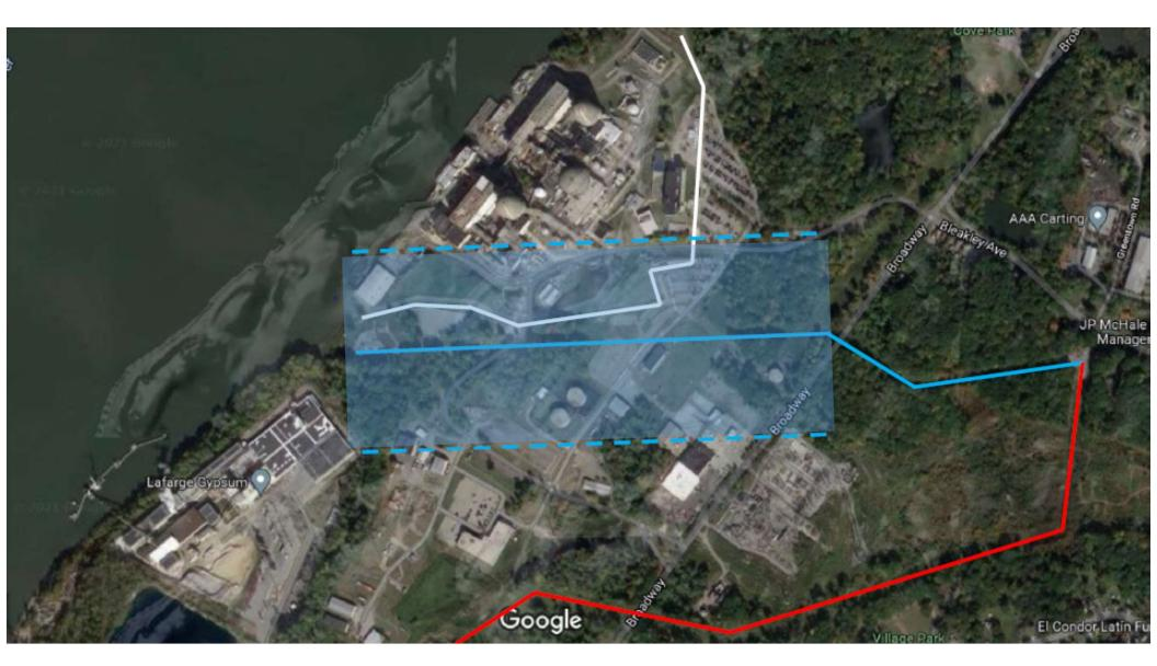
The potential impact radius shaded in blue indicates an area where rupture of the natural gas pipeline could damage structures in the zone.
